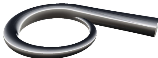
3D CAD model for an asymmetric volute as output from TURBOdesign Volute
